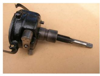
The replacement of worn distributor bushes can present a problem if a stepped removal driving tool is not available. Model A parts suppliers do not sell them. One method to get the bushes out is to screw a 14 mm intermediate tap into one bush as shown in the photograph and using a mild steel or brass rod drive the bush plus tap out from the opposite end. This is then repeated for the other bush.
