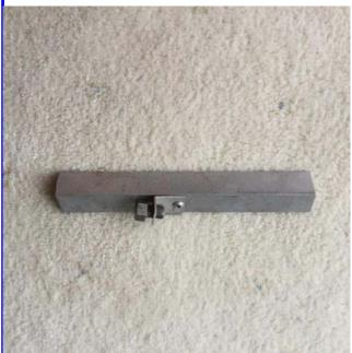
This is the tool that ensures accurate clutch finger adjustment. A piece of 25x25mm angle aluminium cut 210mm long has a bracket to hold a bolt at 70mm from one end. The bolt
