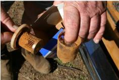
Here is a fuel filter where E10 fuel was left in a vehicle that stood without use for 6-10 months. So change fuel from E10 if storing your vehicle, otherwise
