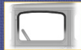
Murray: arched top of door window opening
