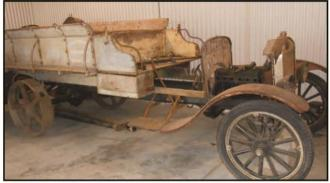
Truck - 1924 Model T original tray/dray style 2 speed tail shaft, 2 speed rear end, cast iron farm rear wheels. Chassis to be restored but not the original timber body with unique signpainting on the side.
