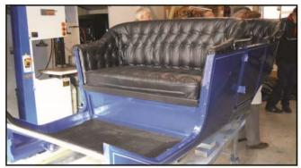
Current Restoration - 1912 Model T Tourer Steve rebuilt the timber frame using the original as a template. Repaired rusty panels, painted and hand pinstriped the body, beautifully upholstered the two bench seats. All wheels retimbered. Front & rear axles restored - seals, bearings, spindles.
