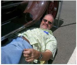
a reconditioned engine fitted plus a new syncho gearbox. The second photo is of Peter Wigzell enjoying a sun bake whilst at the same time tightening the Pitman arm bolt and thereby taking some of the slop out of his steering. Roz had the good sense not to come.
