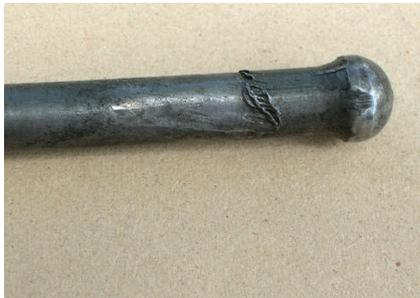
This photograph shows one end of a front brake operating pin which has suffered scoring by rubbing on the inside of the king pin. It has occurred due to the brake actuator arm not being full engaged with the cup on the top of the king pin. (Refer to the figure below). The cause can be due to a number of things such as:
