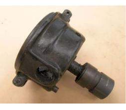
force that the distributor body broke in two as shown in the photograph and required replacement. If this had happened far from home I would have been in serious trouble without a spare distributor.
