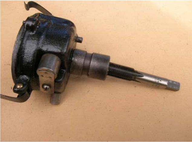
The replacement of worn distributor bushes can present a problem if a stepped removal driving tool is not available. Model A parts suppliers do not sell them. One method to get the bushes out is to screw a 14 mm intermediate tap into one bush as shown in the photograph and using a mild steel or brass rod drive the bush plus tap out from the opposite end. This is then repeated for the other bush.
