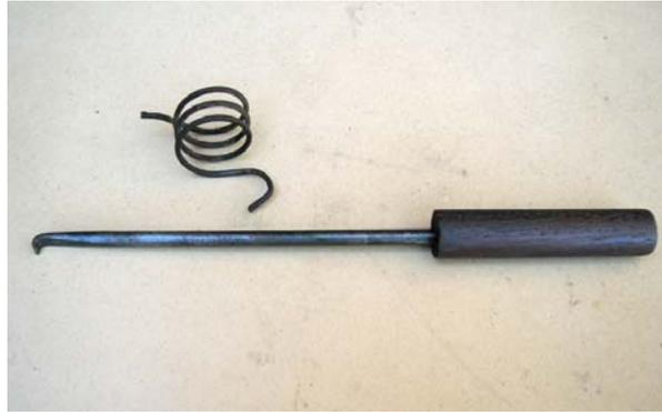
the bent end of the spring and is pulled into the required position on the operating lever.
