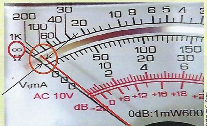
A cheap OHM meter will do this test. When test leads make contact, in either test, the needle will move quickly from the "infinity" setting (black needle) to *almost* the 200 (+-) mark (red line) and then fade back to "infinity" (∞). If ∞, condenser should be working. If no movement or a higher steady setting is read, the condenser is trash. (CY)
