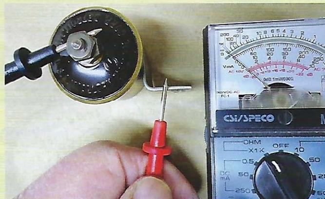
Test 2: Reverse the placement: Attach the black to the hot lead. Touch the red to case.
