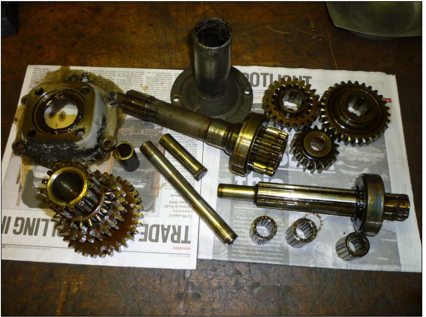
Shown here are all the internal parts of the transmission that have been removed.
