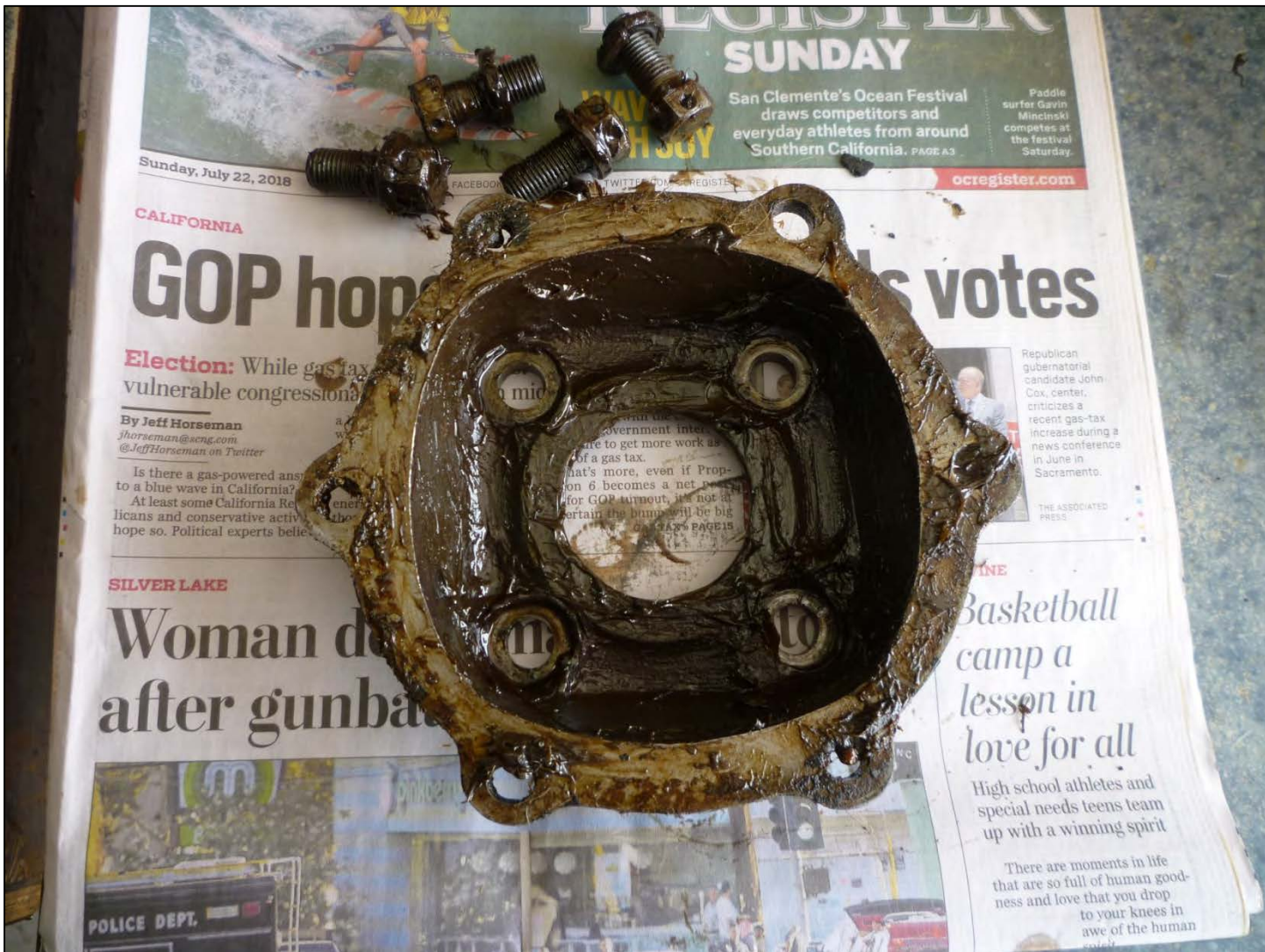
The rear bearing retainer and the four bolts are shown removed.
