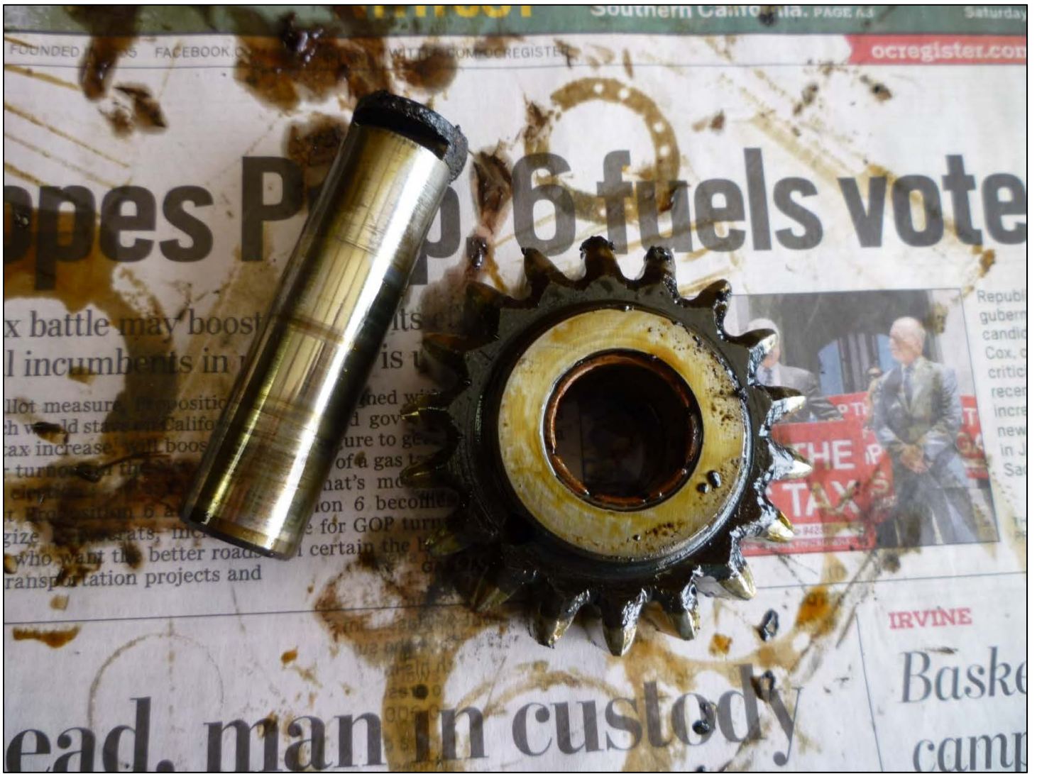
Shown here is the removed reverse idler gear and the shaft.
