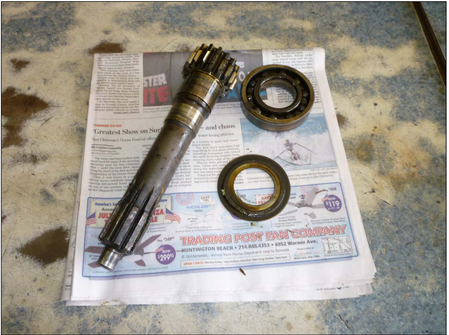
Shown here is the input shaft and the front ball bearing after it was pressed off the shaft. Also shown is the front bearing oil baffle that installs between the bearing and the gear end of the shaft.
