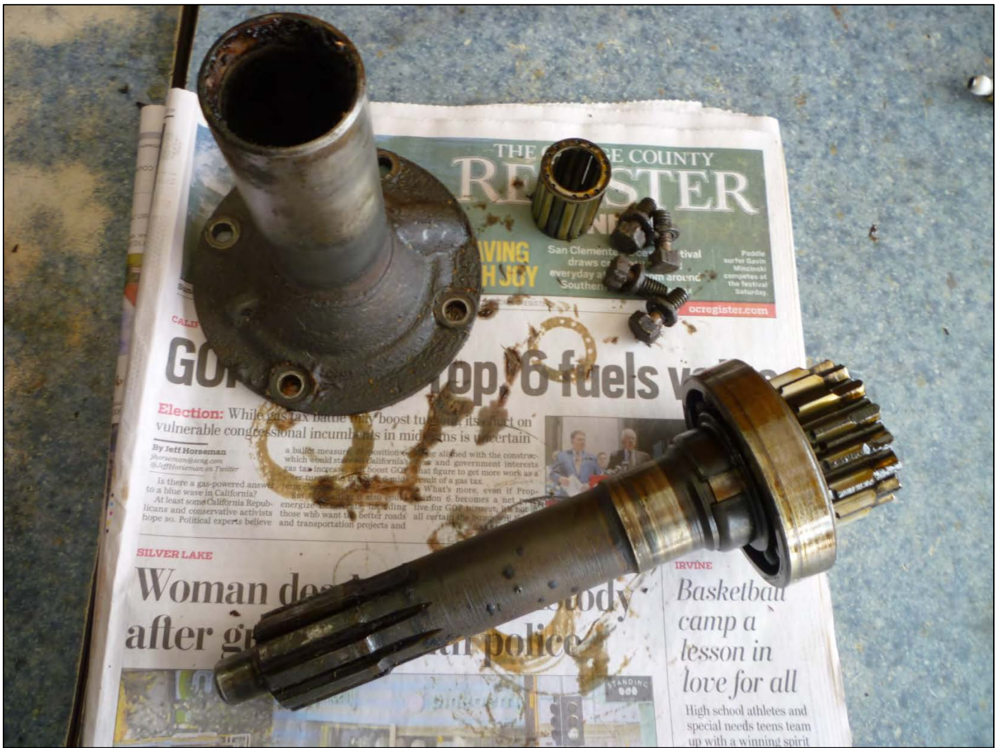
Shown here is the removed front bearing retainer, the roller bearing, and the input shaft.
