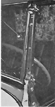
This very desirable accessory folding windshield stanchion permits the windshield to be folded flat on the cowl.
