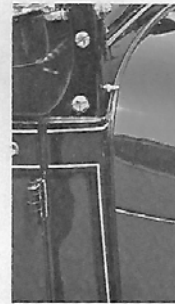
Shown for comparison is a standard 1929 windshield lower section. Note similarity to the accessory frame in that area.
