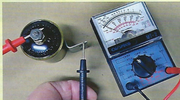
Test 1: Attach the red lead to the hot point on the condenser. Touch the black lead to the metal case on the condenser.
