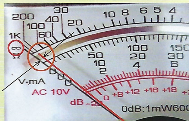
Test 2: Reverse the placement: Attach the black to the hot lead. Touch the red to case.
