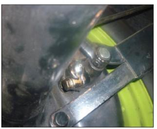
The above photo shows a grease fitting in service on a vehicle driven daily. Give it a shot of grease whenever greasing the car.
