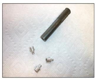
Press in type grease fittings and the insertion tool
