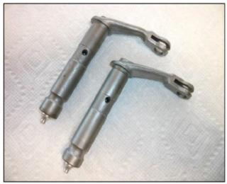
The above photo shows a pair of brake levers with grease fittings installed. Drill from the end of the shaft with a nominal 1\8" drill bit down to a point between where the two bushings ride and cross drill it. Then drill the end of the shaft with a 5\16" drill bit about 3\8" deep.
