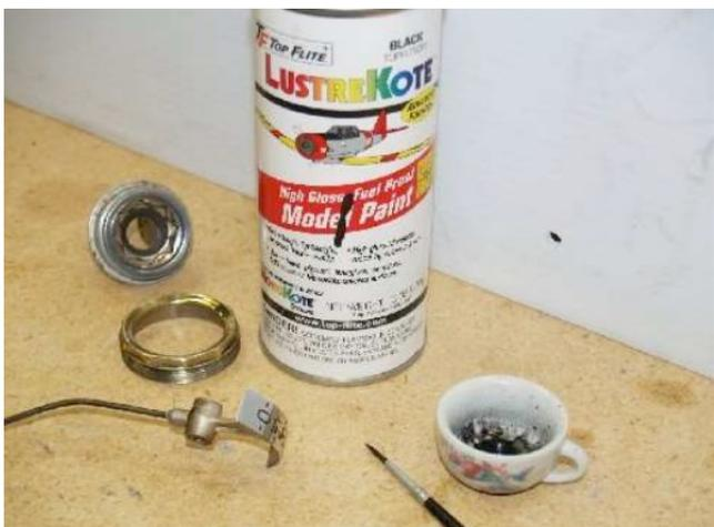
Getting just a bit of paint on the tip of the brush, I let the paint flow into the recesses of the numbers where they had been chipped or eaten away over the years.
